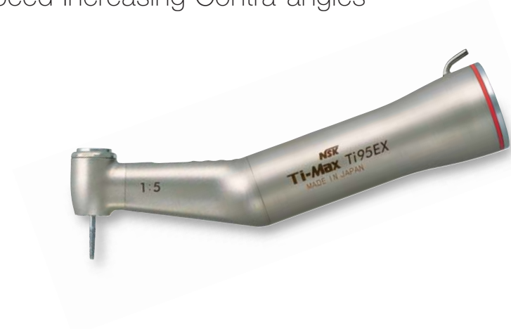
MODEL Ti95EX ORDER CODE C487 • Solid Titanium Body • For FG burs • Max. 200,000 min -1 • Ceramic Bearings • Clean Head system • Ultra Push Chuck
